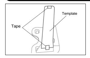
1. Align the template with the outer circumference of the accelerator pedal and attach.
